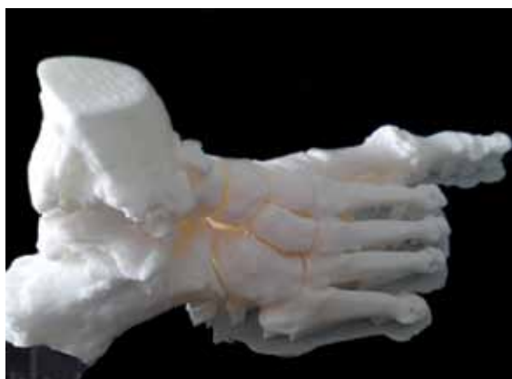
Fig. 1: A 3D printed model of foot based on the CT scan images of the foot
